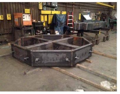
The central (middle) octagonal tube steel ring, located at the top of the dome.
