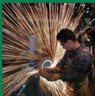
The mirror finish requires 12 to 14 hours of grinding and polishing for each square foot.
