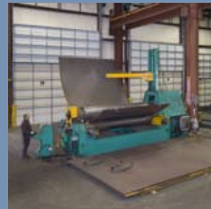
Chicago Metal Rolled Products can curve plates 12 ft-wide and 2 in. thick.
