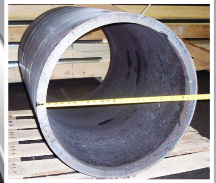
1½" plate 45" long rolled to a 25" inside diameter
