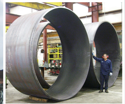
2" x 58½" beveled plate rolled to a 128" outside diameter
