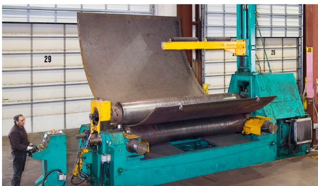
2" x 12' plate roll can roll 40ft lengths
