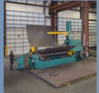
Chicago Metal Rolled Products can curve plates 12 ft-wide and 2 in. thick.
