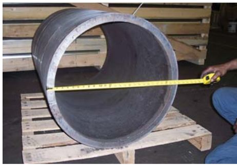
1-1/2" plate 45" long rolled to a 24" inside diameter
