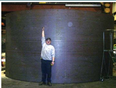
Beveled 5/8" plate x 115" long rolled to an 11' diameter in 180 degree segments
