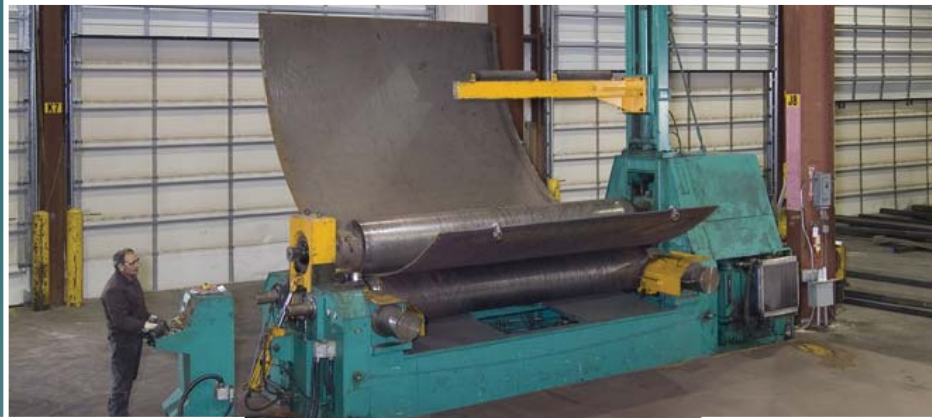
2" x 12' plate roll can roll 30' lengths
