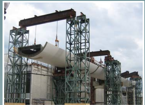
5/8" x 12' wide 20' long with a 10' radius for a bridge at Chicago's Millennium Park
